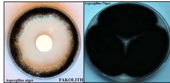
Aspergillus Niger culture, and the inhibition halo of BioFilmStop technology.
